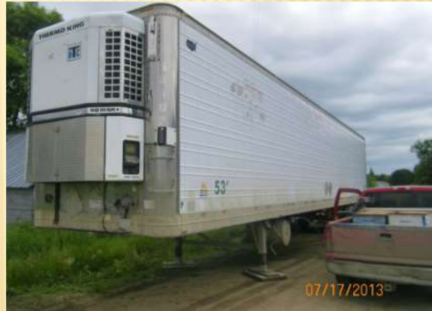
Steppler Farms uses a reefer. This trailer is cooled to 20F for a week to freeze out the wax moth.
