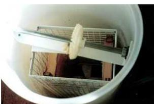
The frames of honey with the cappings removed are then placed in a machine like a spin dryer. The combs are seen in the photograph left, placed vertically in a wire mesh basket inside the drum of the machine. The basket then spins around rapidly on its vertical axis, either turned by hand or by an electric motor. As the combs spin round rapidly, the honey flies out of the open wax cells, strikes the wall of the drum and trickles slowly down to the reservoir at the bottom.
