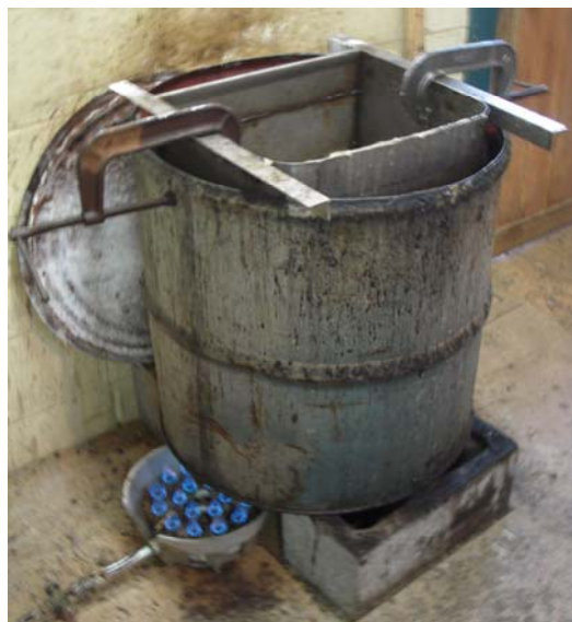
Steel tank in a drum with water heated by a propane burner.
