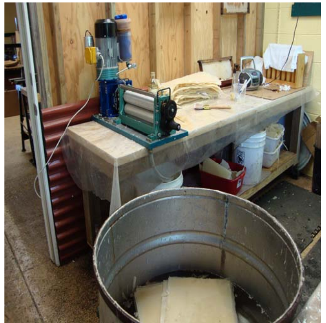
Wax sheets are placed in warm water sump (80-85 degrees) so they will not be brittle when running through the embossing machine.
