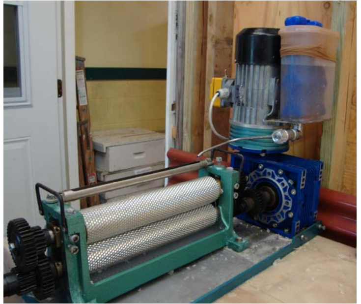
Embossing Mill– the mill can be ordered with different size embossing rollers and flat rollers as well.
