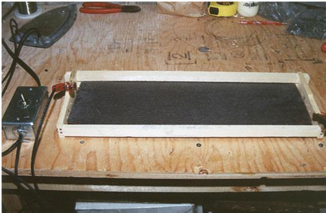
Place the electrical clamps on the wire at each end. insert a piece of wax foundation into the top groove, laying on top of the wires. Give the wire a few seconds electrical charge. You will see the wires start to melt right into the wax.
