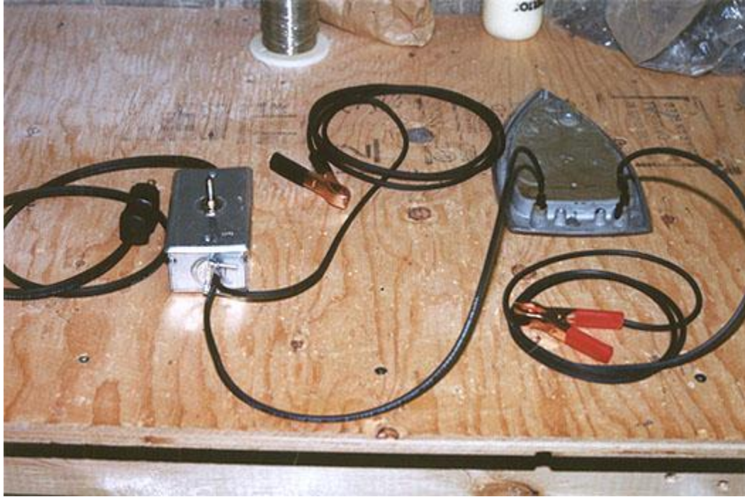
Various contraptions can be made to provide a low current to the wire. Battery charger, transformer, here a clothes iron.
